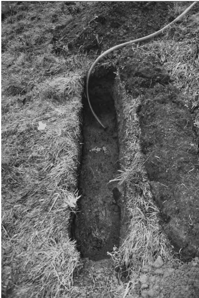
Figure 7.91 Injection of Naphtionate in a trench 18 m uphill the spring Zipfeldobel.
