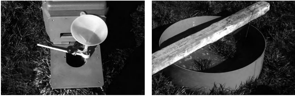
Figure 7.18 Left: Injection equipment consisting of cone and fixed hose introduced in the 4 in.-well; right: Injection of concentrated Uranine solution in a filtration pool.
