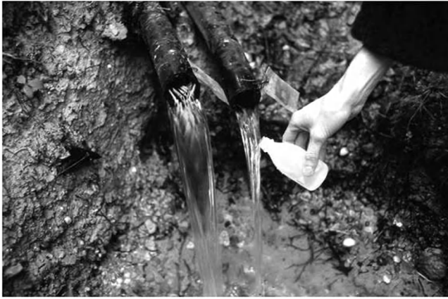
Figure 6.2 Sampling to assess the levels of environmental tracers and to determine the background concentrations of the artificial tracers to be used.
