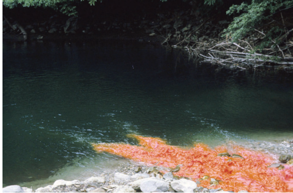
Plate 5a: Situation 10.23 a. m.: Injection of the small river. Start of stratification in the lake water body in the depth determined by the density.
